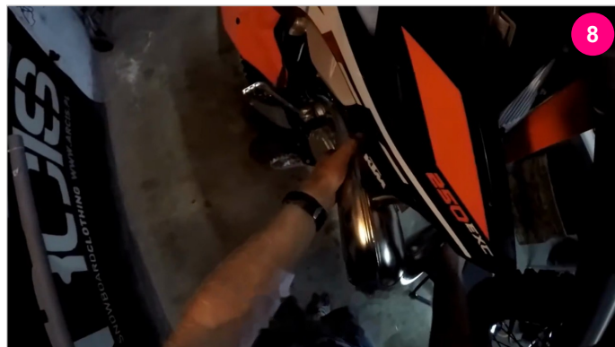
INSTALL THE PIPE
