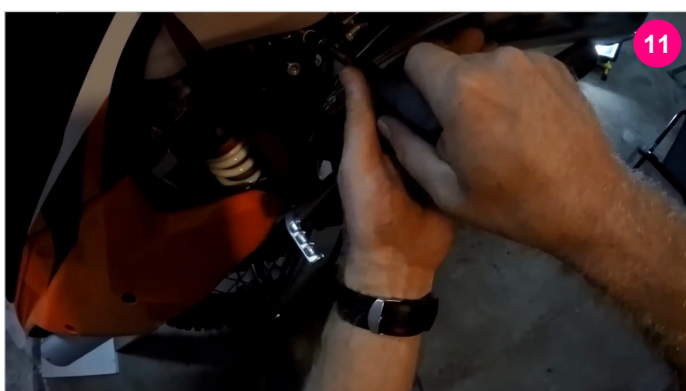
TIGHTEN THE PIPE SCREWS
