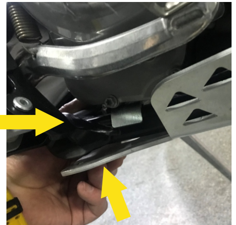
DPRESS THE REAR PART OF THE GUARD TO THE FRAME
