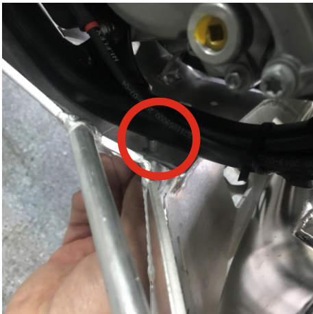
GRIP SCREWS TO FRAME SOCKETS
