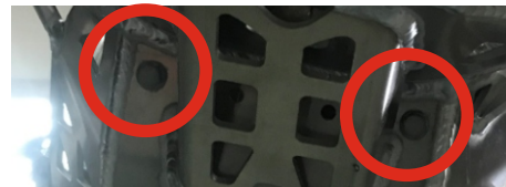
DPRESS THE REAR PART OF THE GUARD TO THE FRAME
