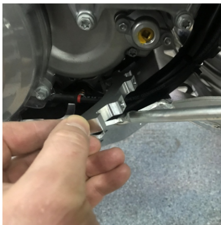
PUT THE LEFT HANDLE AND SCREW THE SCREW
