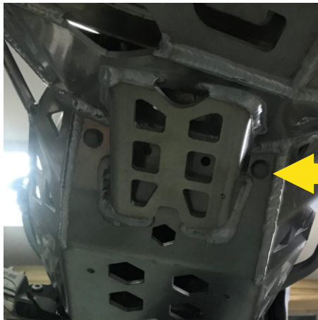
TIGHTEN SCREWS SEVERAL ROTATION
