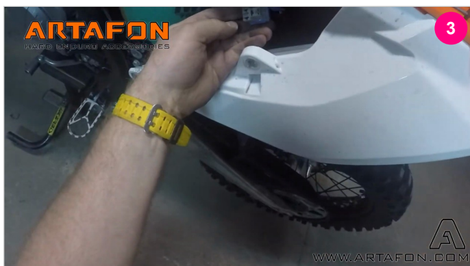
TAKE OFF RUBBER PAD FROM PLUG
