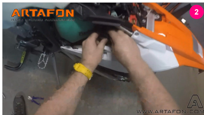
TAKE OFF THE FIRST PLUG (BLINDED WITH RUBBER PAD)
