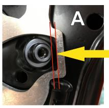
SPACE BETWEEN THE GUARD AND THE RADIATOR MOUNTING ON FRAME FOR PLASTIC FITTING OF THE RADIATOR
